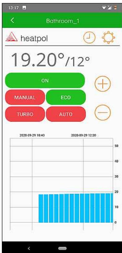
The first temperature ( 19.20° ) - is measured with the remote / temp. sensor (H+R). This is the actual room temperature. The second ( 12° ) is the temperature set for the room.
